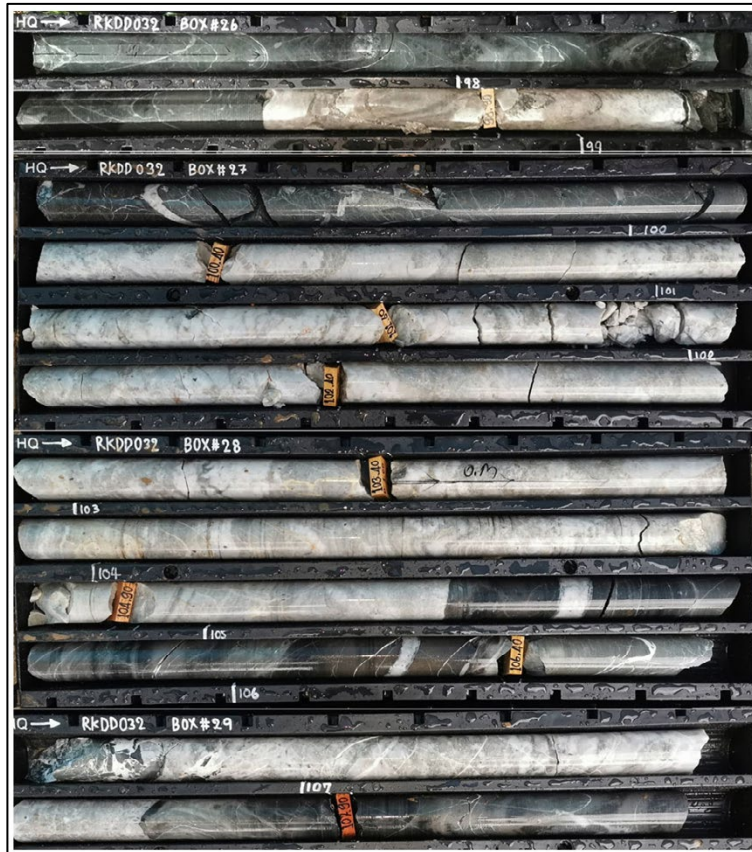
Photo 4. RKDD032 from 97.4m to 108.2m, showing pegmatite swarm with pale lepidolite.
