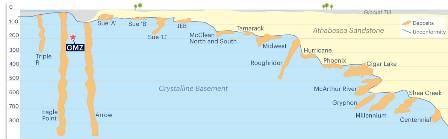
Image: Schematic of Athabasca based deposits, basement hosted versus unconformity, and inferred position of Gemini Mineralised Zone in the model.
