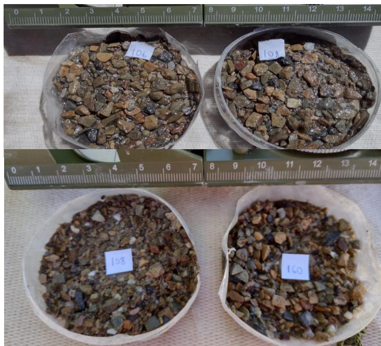
Figure 2: Cuttings of drill hole PB-01-21. These are cuttings of a polymictic conglomerate which we now know to extend through a min 40m zone of no recovery from the previous adjacent drill hole PP-01-19.
