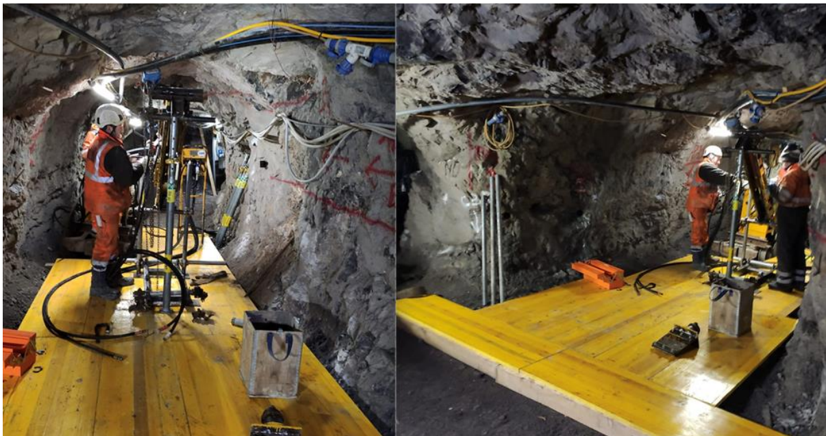
Figure 2: Diamec-230 Drill Rig Underground at Ponente
