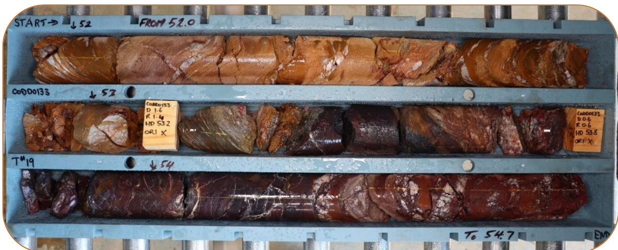
Figure 4 – Codd0133 52m to 54.7m showing purple-red gossan from 53.3m
