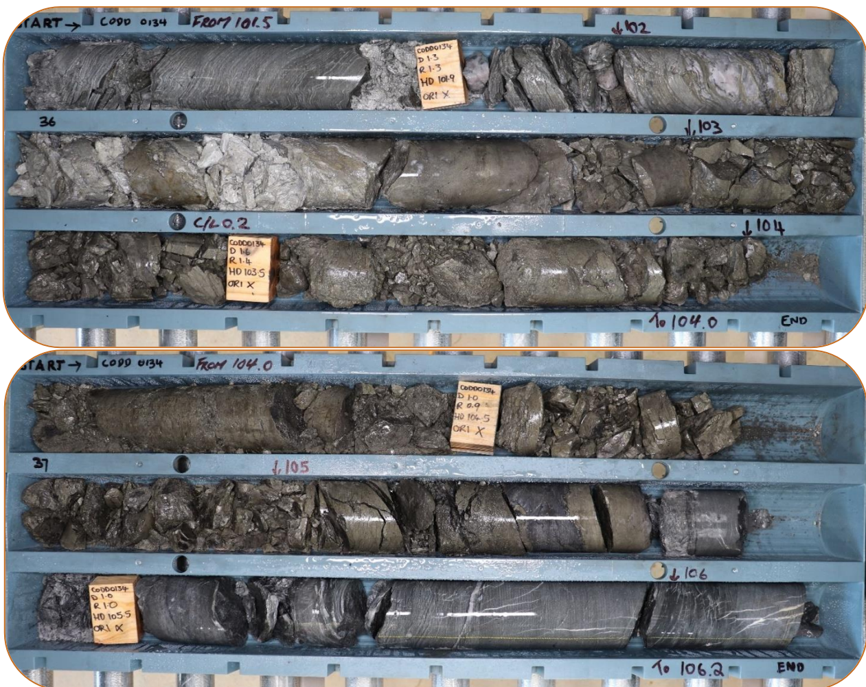
Figure 5 – CANDD0134 101.5m to 106.2m showing massive sulphide from 102.3m to 105.5m comprising stratiform fine-grained pyrite and chalcopyrite
