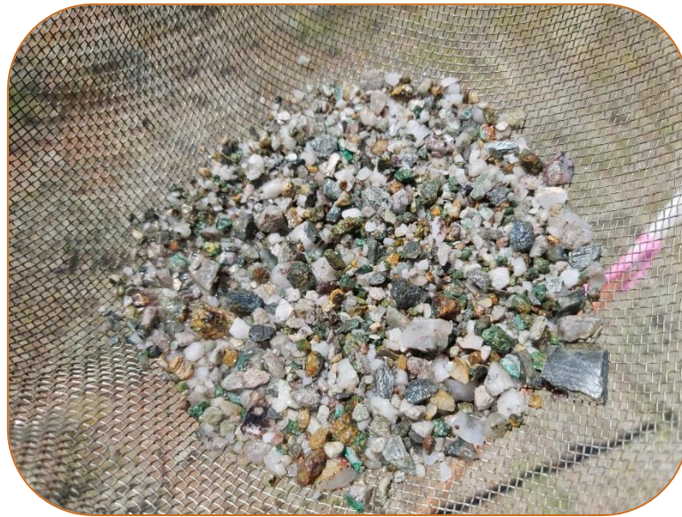
Figure 7 – Copper oxide mineralisation; malachite and quartz in CORC0139 at 35 metres.
