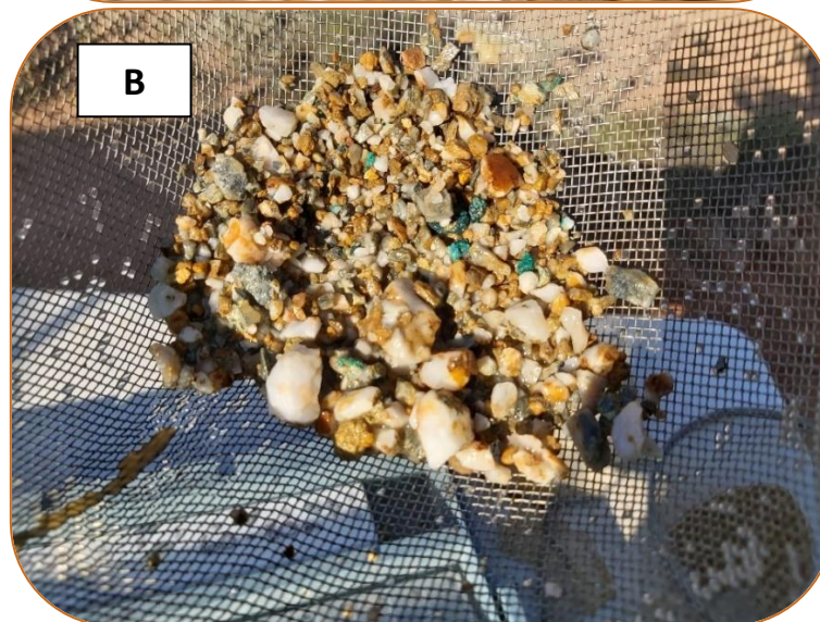
Figure 8 – Copper oxide mineralisation. A: malachite, azurite and quartz in CORC0141 at 38m. B: malachite and quartz in CORC0144 at 39m.
