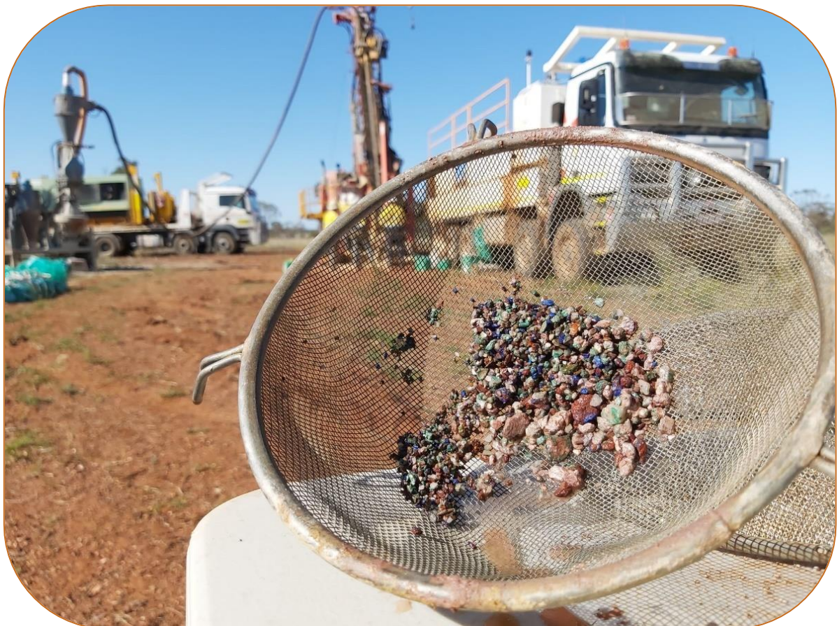
Figure 1 - Copper oxide mineralisation; azurite (blue) and malachite (green) in CORC0140 at 34 metres
