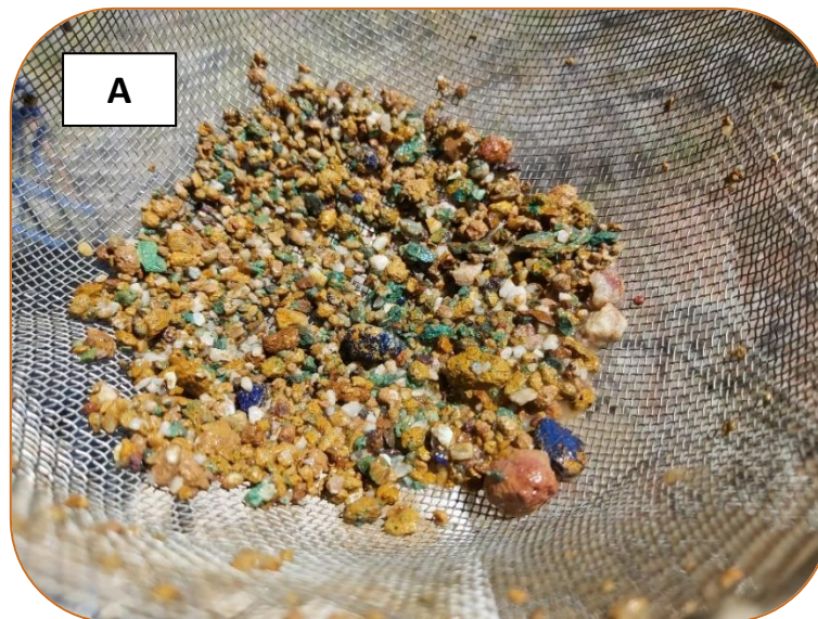
Figure 7 – Copper oxide mineralisation; malachite and quartz in CORC0139 at 35 metres.
