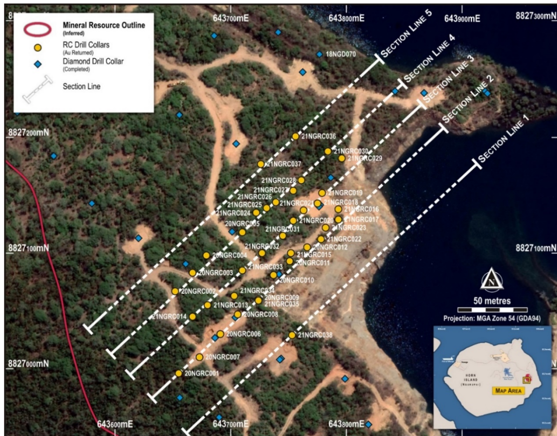
Figure 2 - AQX RC Infill program and diamond drill hole collar locations adjacent to the historic 1980s gold mine open cut pit area.
