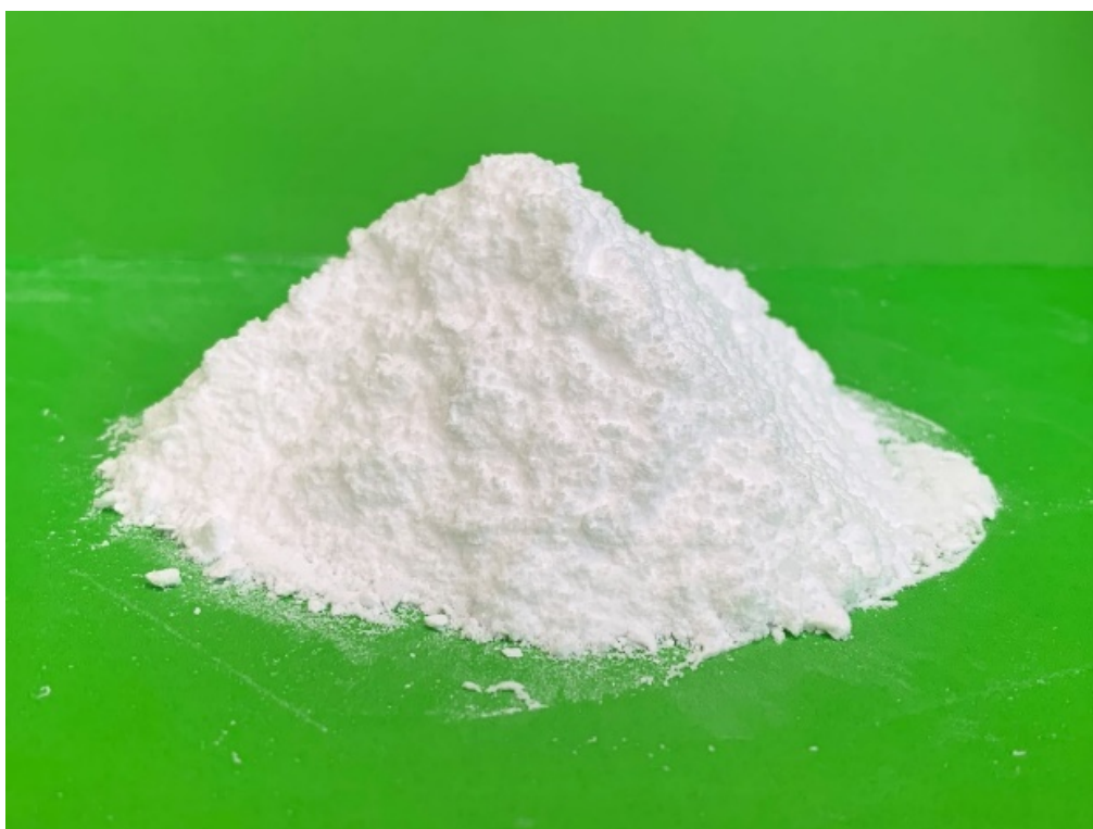
Figure 2: Primary Lithium Sulphate produced from Roche Dure SC6 under metallurgical testing for AVZ’s planned Manono Lithium Sulphate Plant
