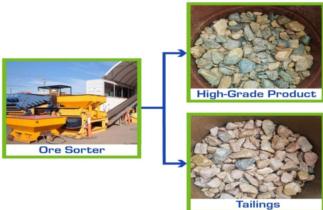
**Image 4: ROM feed to the ore sorter before separating into product and tailings**
