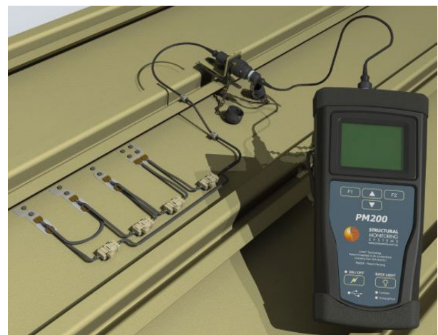
CVM™ Sensor connected to a vacuum source with an accurate flow meter
