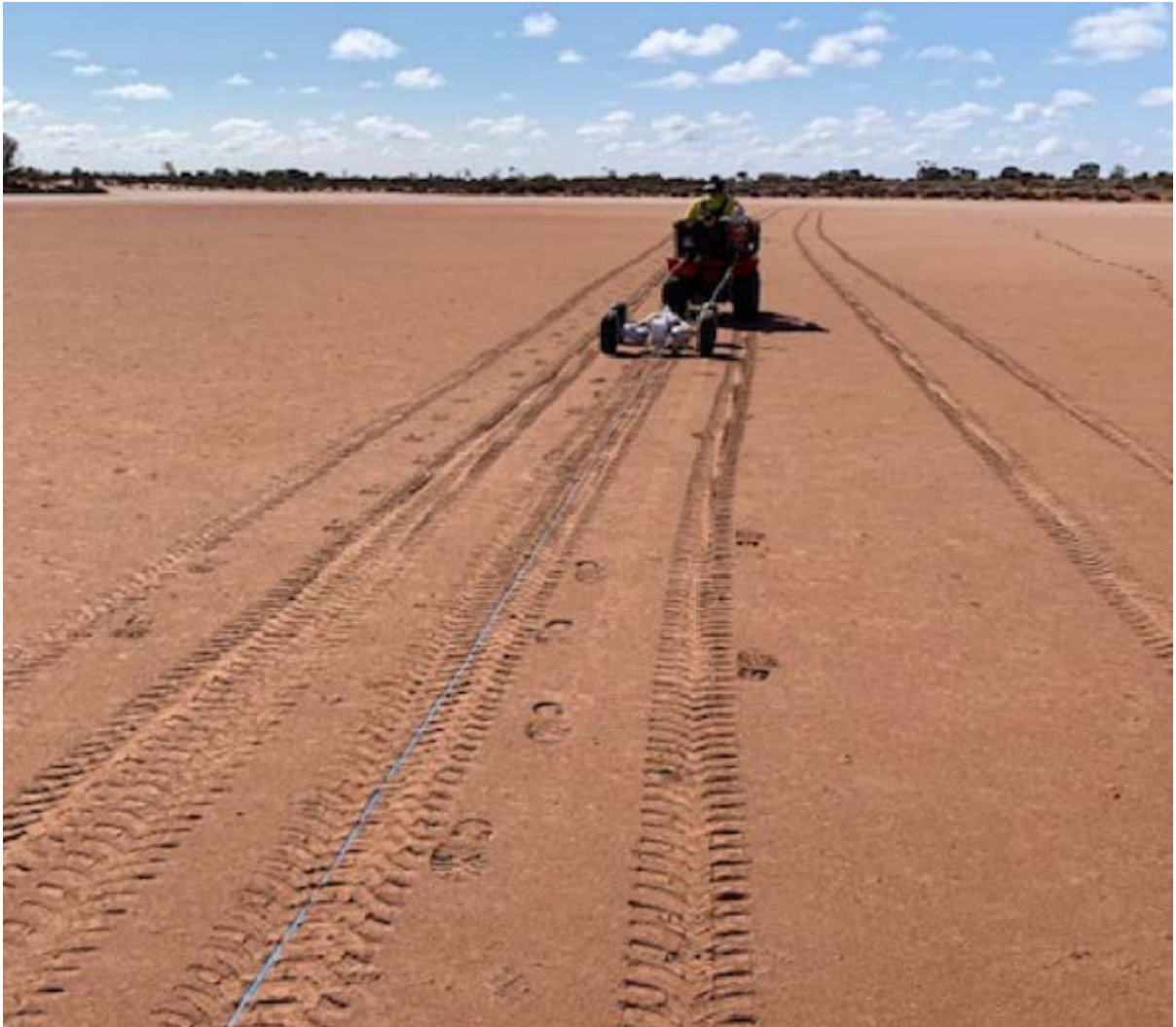
Helical cable ploughed with bob cat dedicated attachment into ground for seismic surveys
