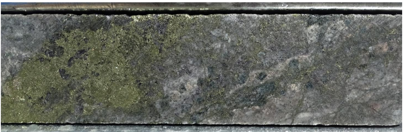
CRP00134D (528m depth down-hole) – 1.8% copper, 0.8g/t gold, 2.8g/t silver and 228 ppm molybdenum. Early-stage porphyry, sericite-chlorite-biotite alteration with 5% A-B vein abundance
