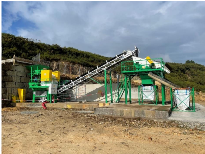
Figure 1 - Pilot Plant Crushing Circuit (Stage 1)
