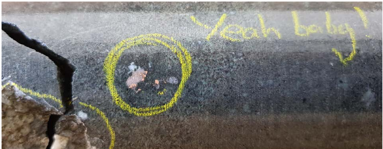
Figure 6 Coarse grained native copper associated with quartz infill in a vesicle in andesite. 109.15m down-hole depth in drill hole CD21-006
