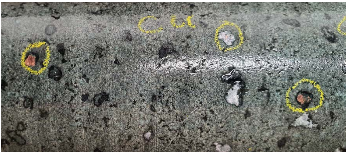
Figure 1 Native copper mineralisation in vesicle infill within porphyritic andesitic-basalt lava flows, 21.35m depth in drill hole CD21-008. Core is approximately 6cm in diameter.
