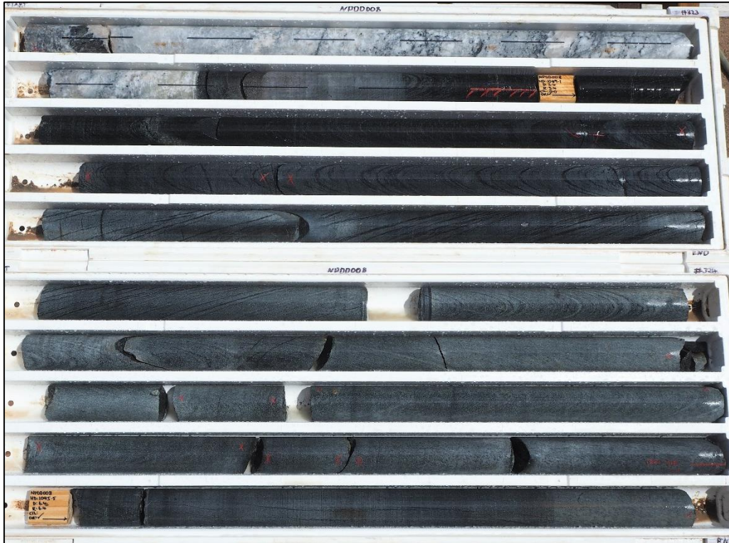
Photograph 1 – NPDD008: upper section of the first of the prospective komatiitic ultramafics (orthocumulates) intersected below the thick pegmatite intrusion (from 1088.5m)
