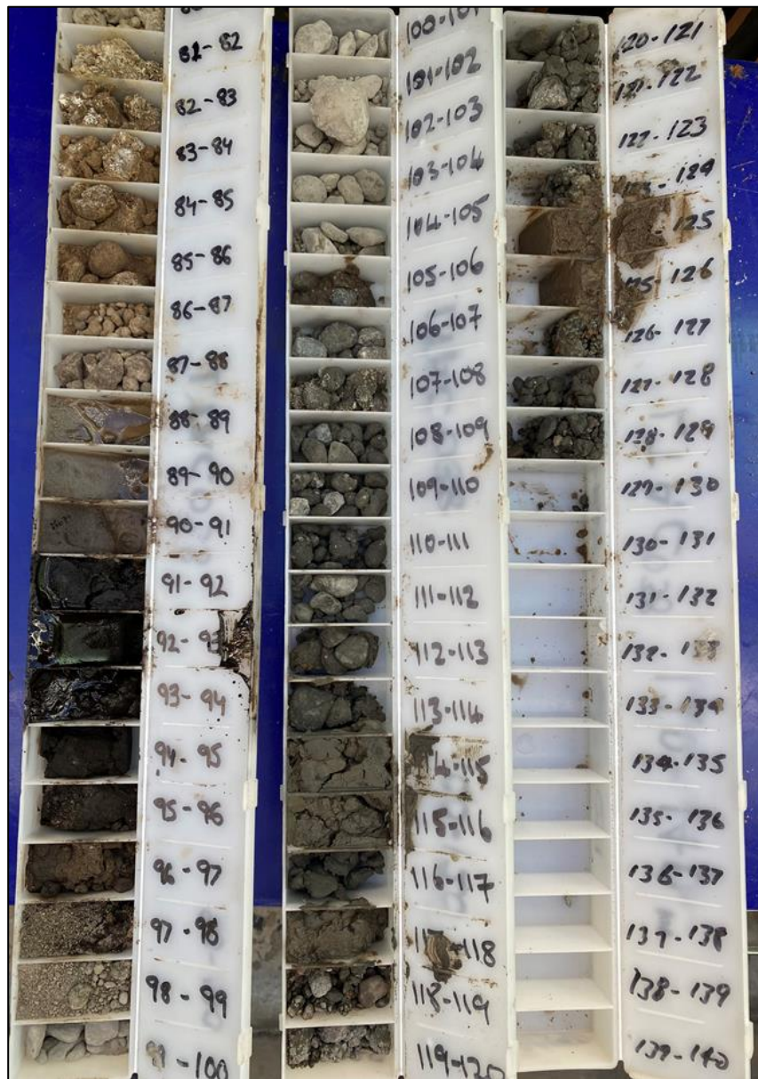
Figure 10: Chip trays showing the basal aquifer sequence (86 to 129m - gravel, fine sand, silt and minor clay)
