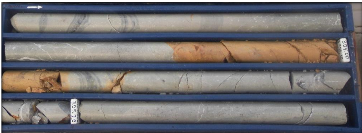
Figure 2a: Core photo RDDH024, interval 302.20m to 305.92m showing an argillic-sericitic porphyry dyke, with quartz veinlets that have pyrite margins. Refer to Figure 1.
