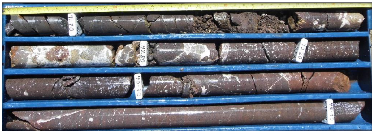
Figure 2b: Core photo RDDH025, 41.5m to 45.2m showing highly brecciated iron-oxide altered andesitic sill with visible malachite (copper) mineralisation.
