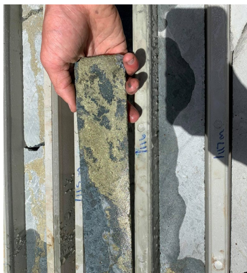
Figure 1: Drill Hole MCDD015 Showing Chalcopyrite Stringer Veins.
