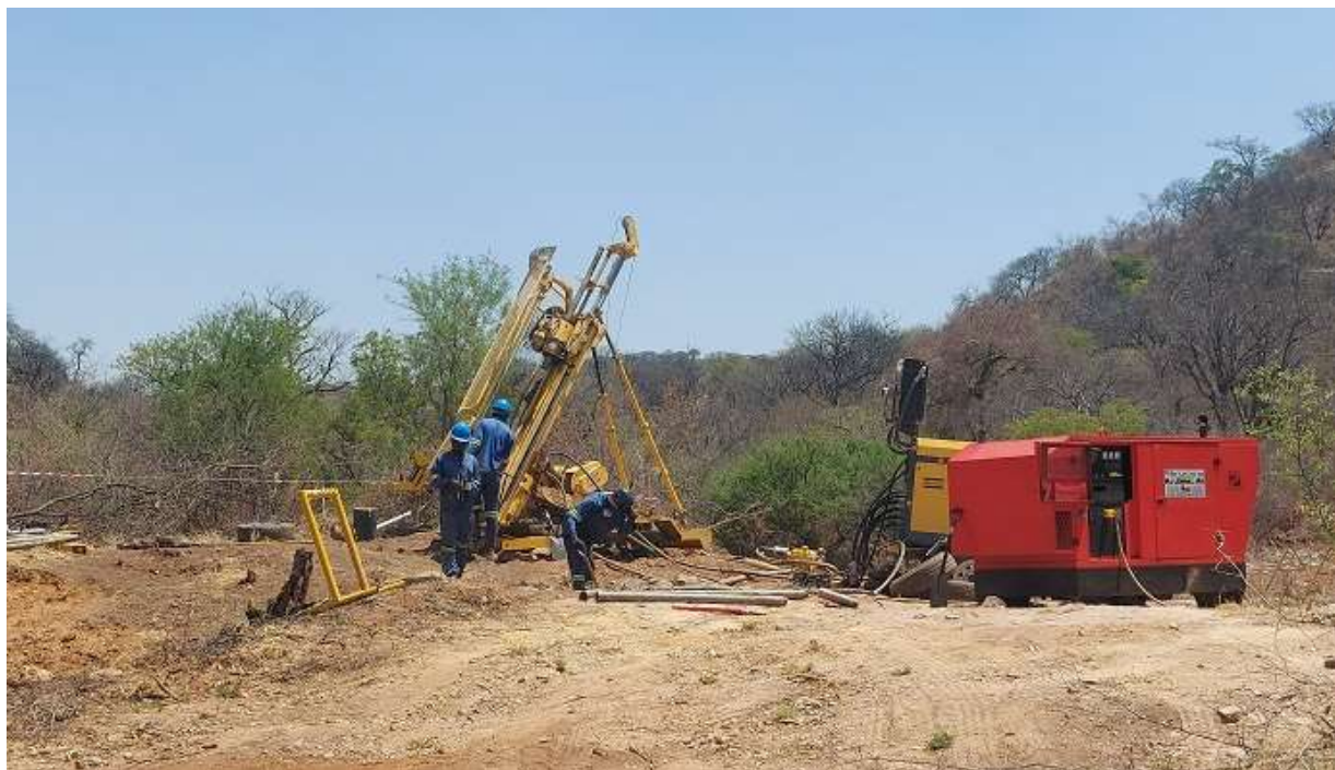
Photo 1: Nosib Block Prospect, man-portable diamond drilling rig testing the shallow Cu-Pb-V zone
