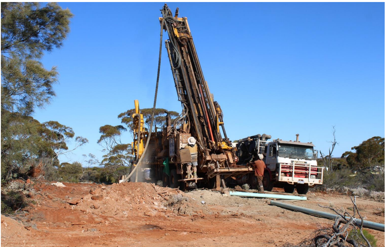
Figure 2; RC drill rig drilling on drillhole VKRC007 testing above hole VDD016 (Figure 3)
