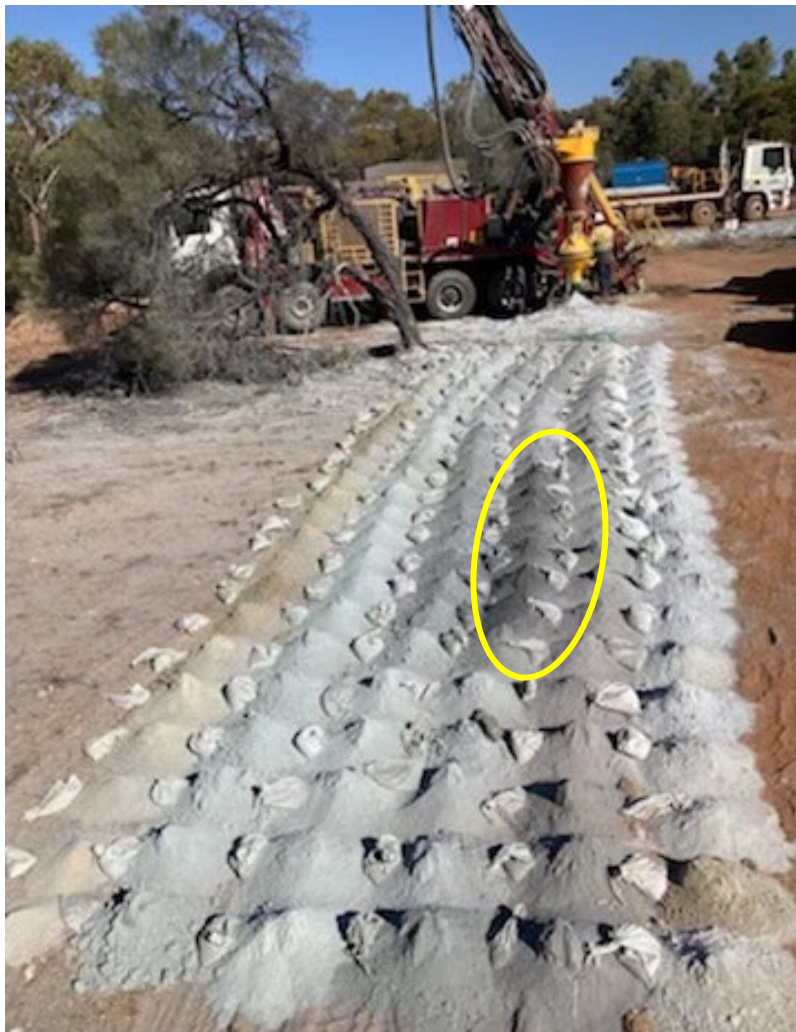
Image: Photo showing RC drill rig and samples from IVRC022 at the Ida Valley Gold Project, ~9m sulphide mineralisation circled
