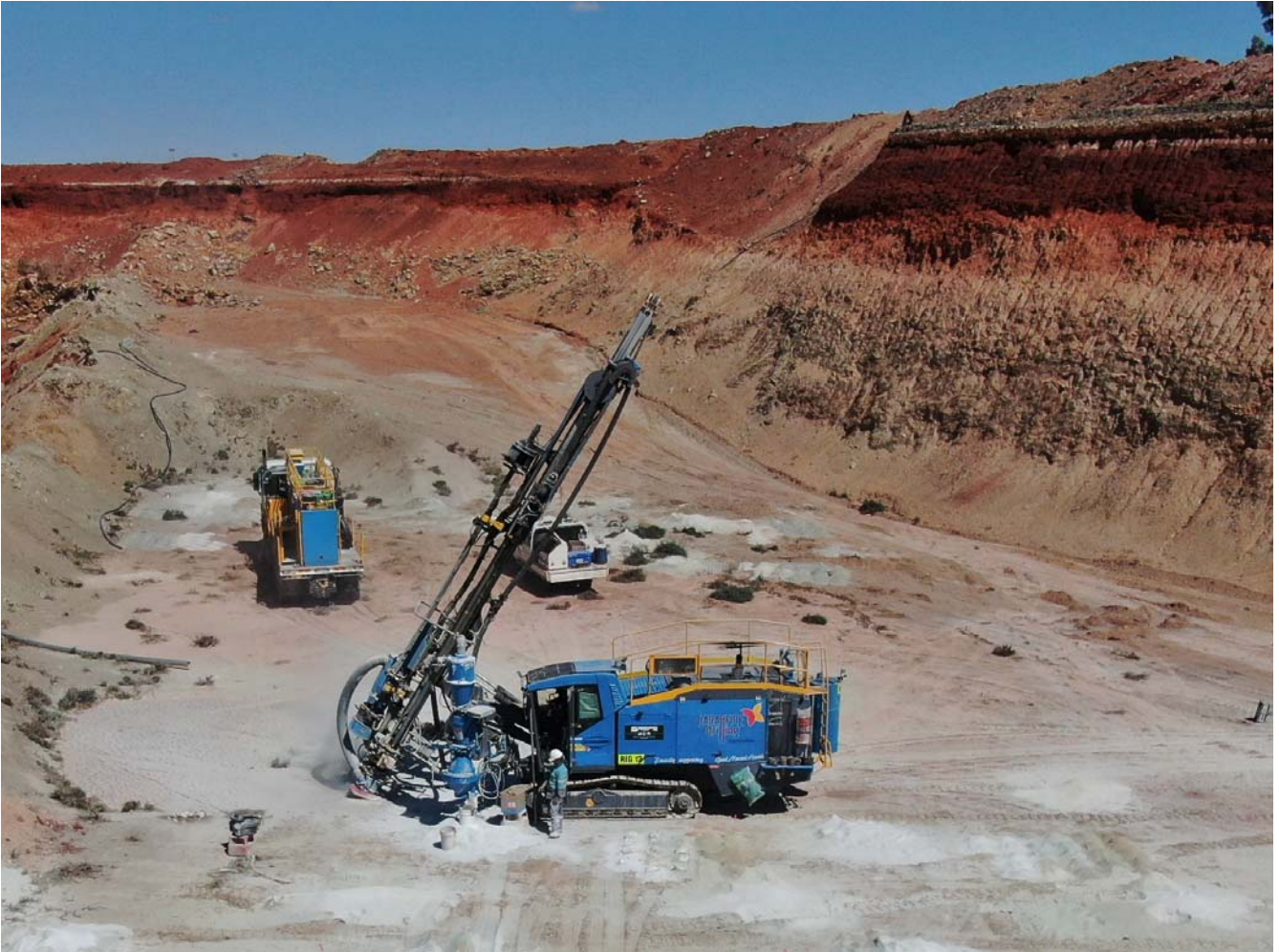
Figure 2: Grade control drilling is being performed by Jarahfire using an Atlas Copco L8 drill rig.
