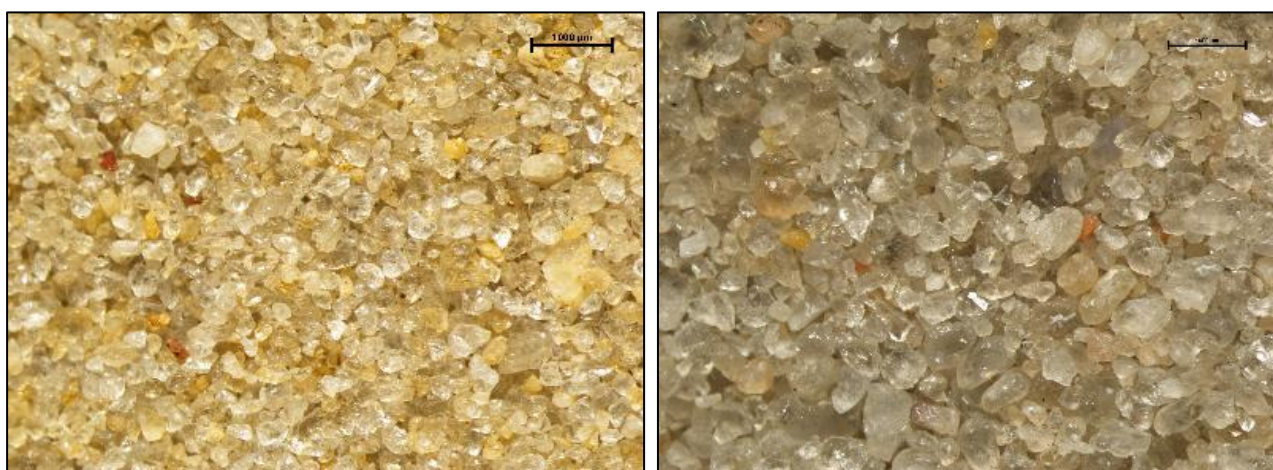
Figure 11: Attritioned HLS SG 2.96 Float Non-Mag -0.6+0.15 mm NVAC004-11-13 (left) and NVAC010-14-17 (right)
