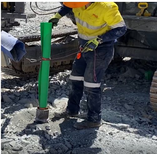
Fig 1. Collar Keeper manually inserted into guide tube
