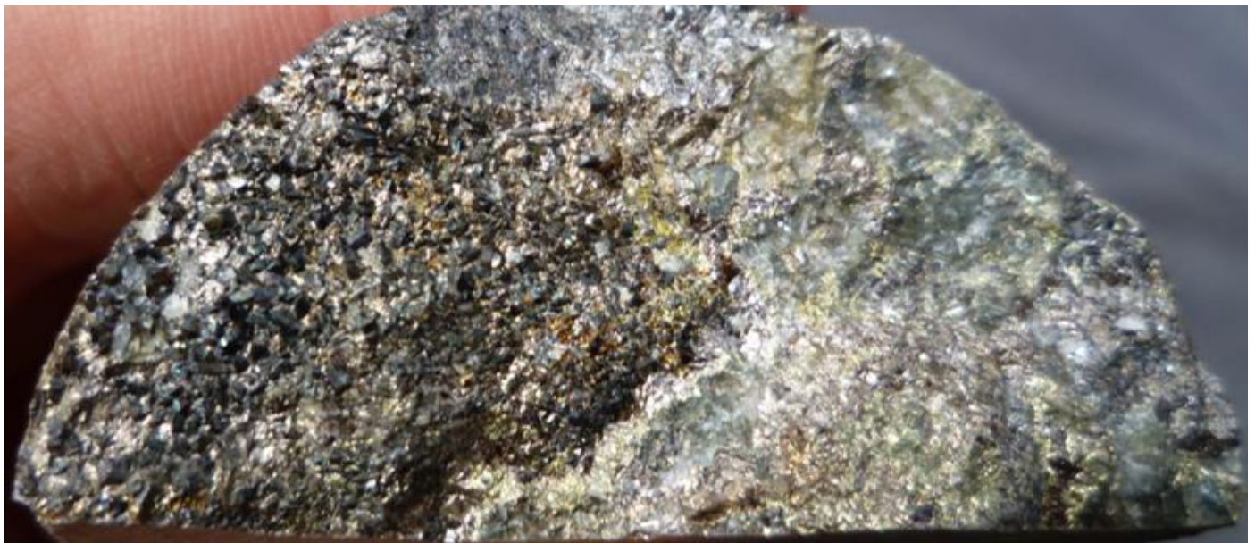
Figure Three | Photo of coarse grained cassiterite on the left hand side, in drill core from 174m in ML134
