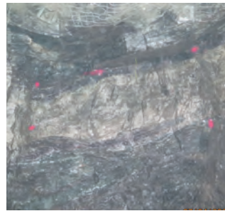
SBA 788 south ore drive (3.5mW x 3.5mH) with a face grade 3.6% Ni
