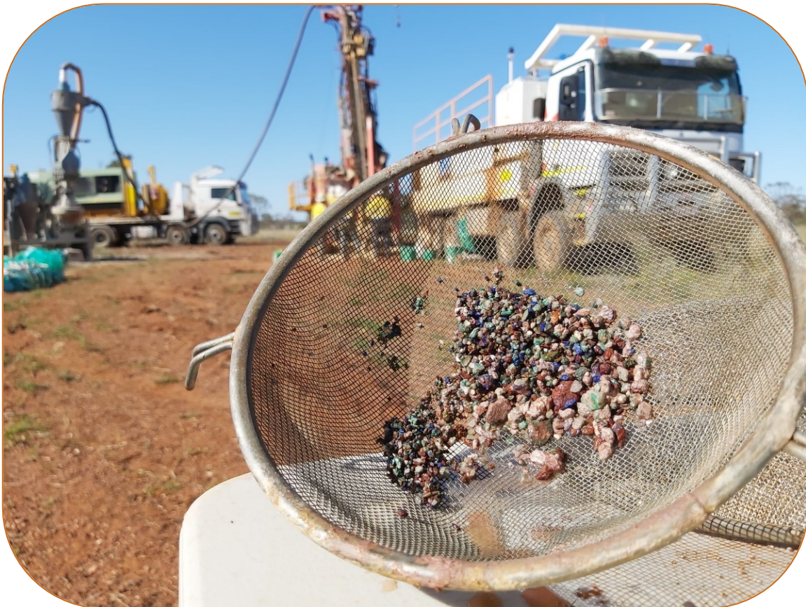
Figure 1 - Copper oxide mineralisation; azurite (blue) and malachite (green) in CORC0140 at 34 metres 2
