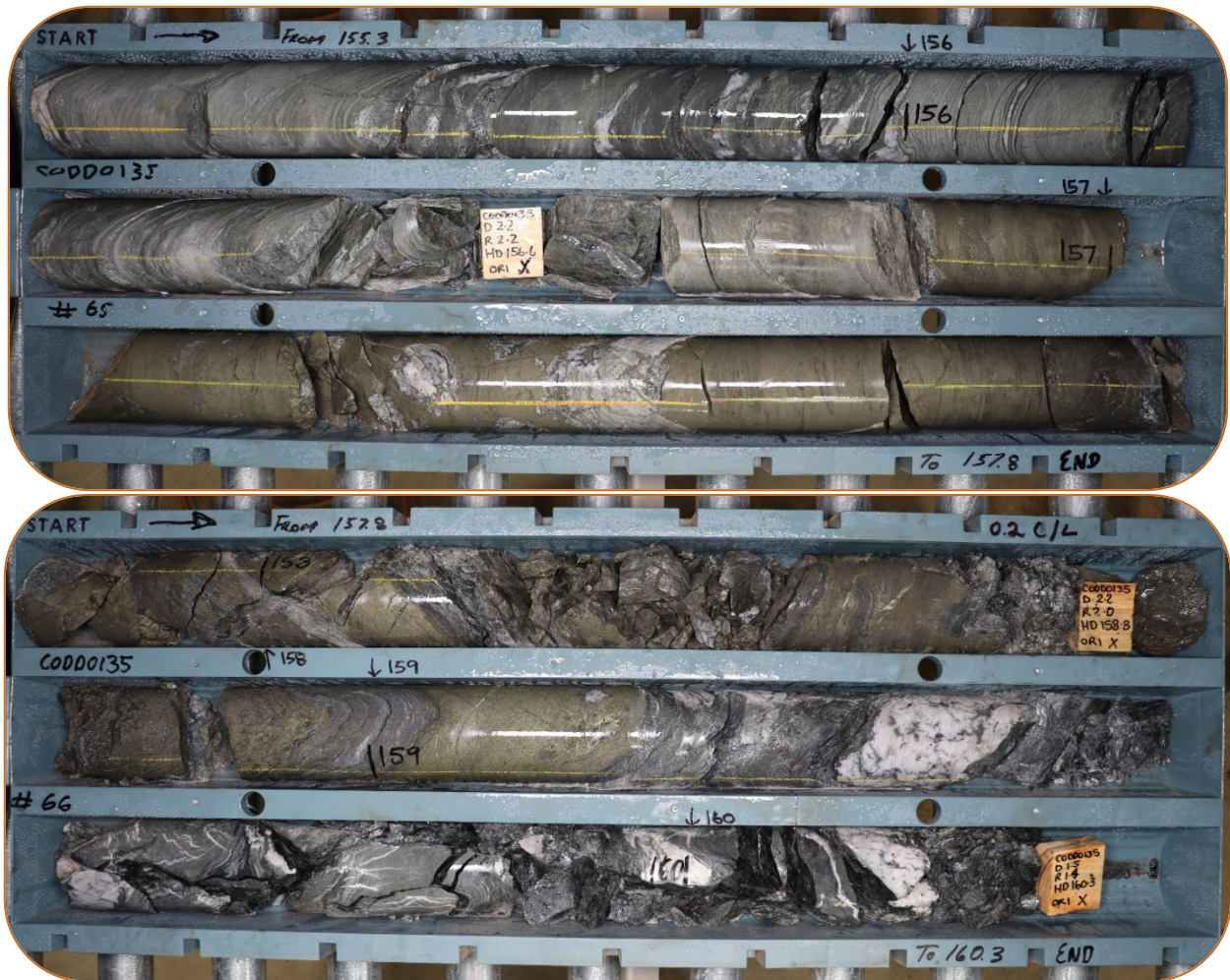
Figure 6 – Codd0135 155.3m to 160.3m showing massive sulphide from 156.8m to 159.2m comprising fine stratiform pyrite with chalcopyrite layers and trace sphalerite.
