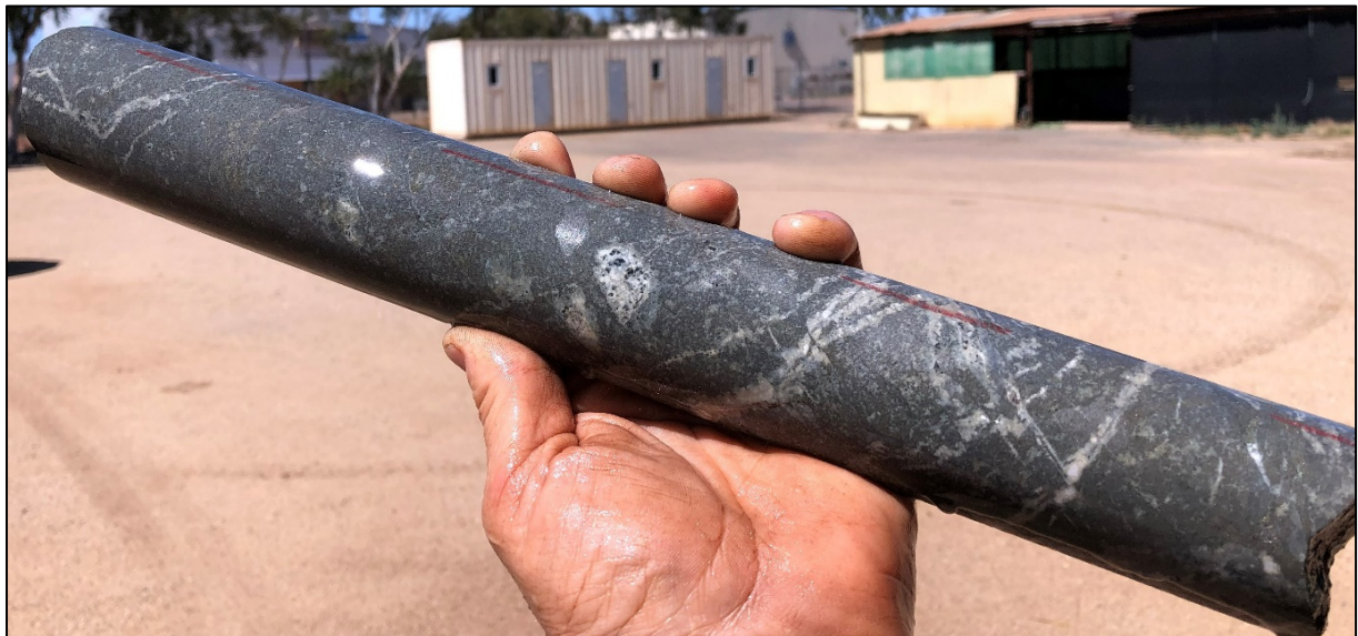
Figure 1. Mineralised drill core from BVD001 – matrix sulphides at 204.5m
