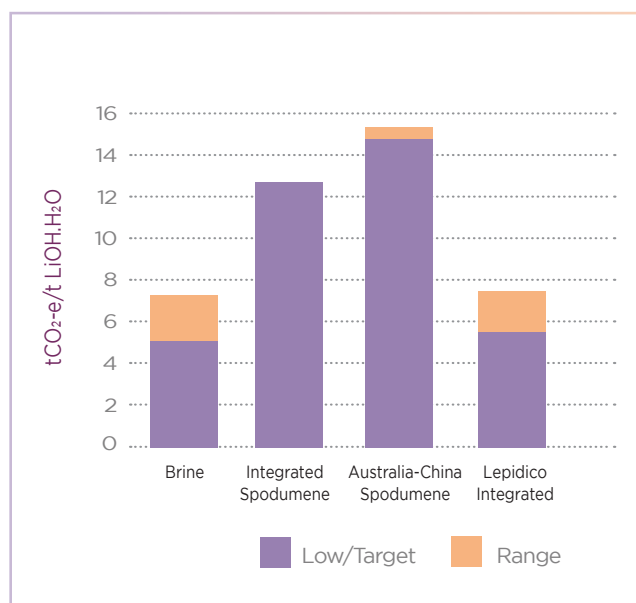
Figure below: CO 2 intensity comparison for lithium hydroxide production tCO 2 -e/t lithium hydroxide
