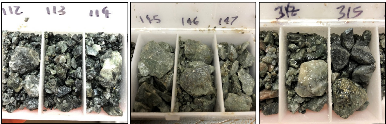
Figure 3: RC drill chip photos for GP01 discovery drill hole 21MYC0245 showing intense intrusion related hydrothermal (calc-silicate and chlorite) alteration of metasediments and associated gold-copper sulphide mineralisation (disseminated and breccia style pyrrhotite and chalcopyrite).
