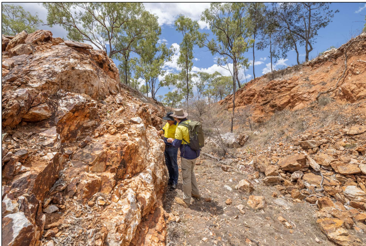
Figure 7. Sunshine Gold's MD, Damien Keys and Exploration Manager, Matt Price, mapping a 1962 costean at Keans. The 4m wide, N-S striking, quartz vein contained abundant fine-grained molybdenite.
