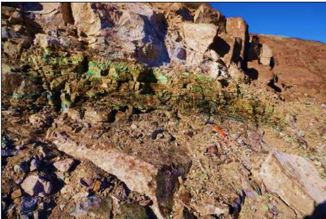
Figure 2: Outcropping visible copper mineralisation exposed in drill pad construction, near planned hole number CMPDD003
