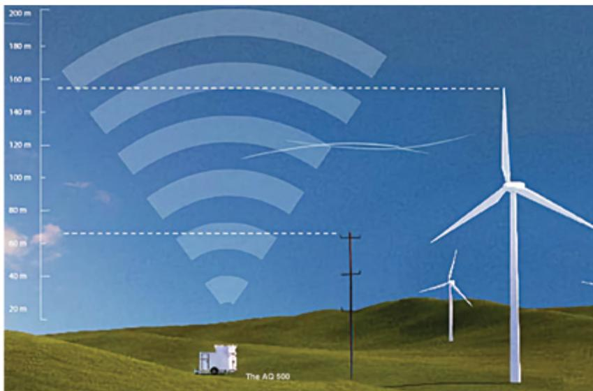
Figure 43: SODAR helps optimize design height for wind turbines.
