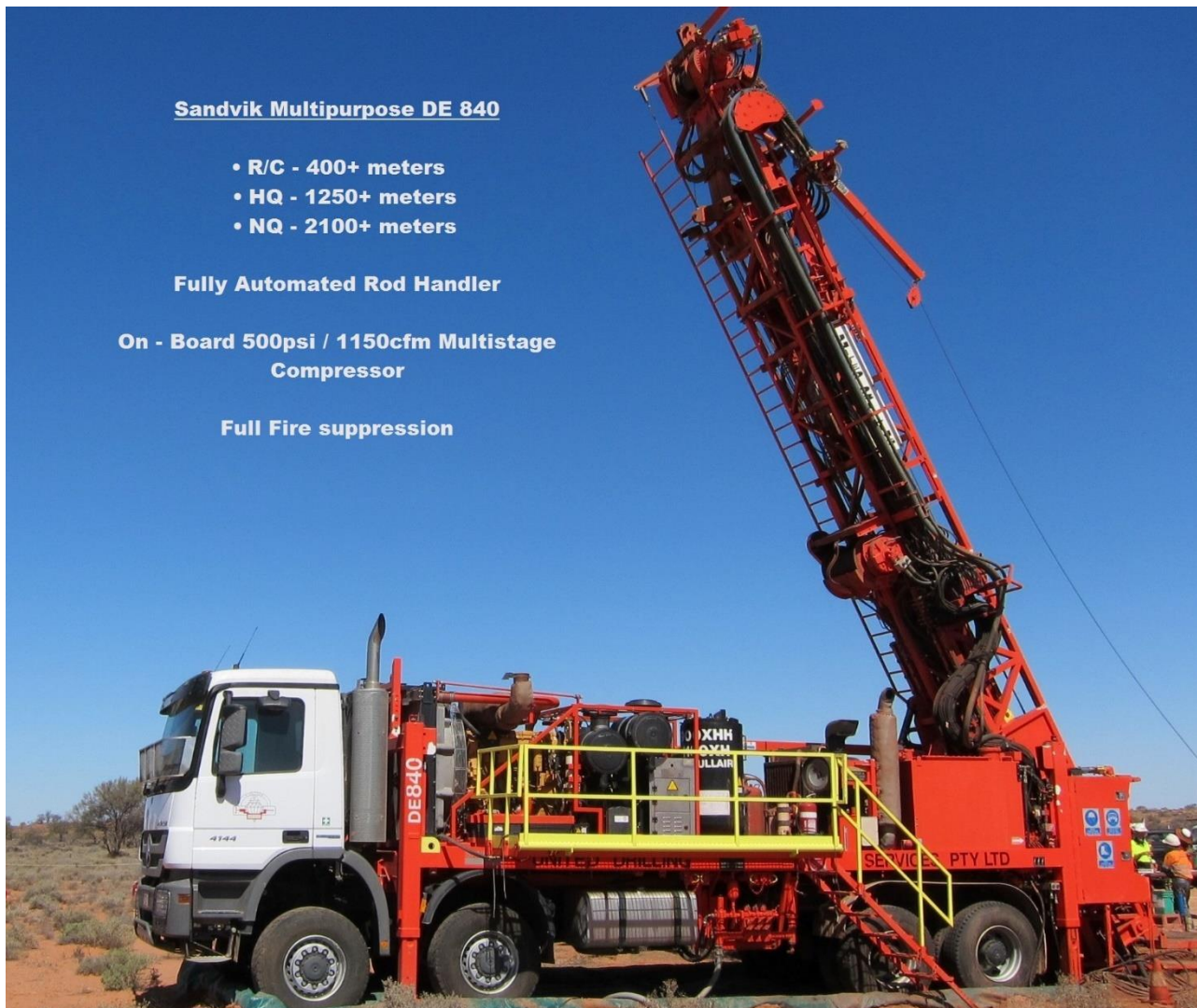
Figure 1: Sandvik DE 840 Multipurpose truck mounted drill rig
