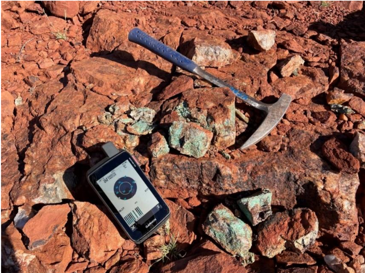
Photograph 5: Malachite-rich sample BLGS0217 (5.73% Cu and 5.74 g/t Au) from infill sampling at Eagles Rest.
