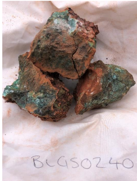
Photographs 1 and 2: Outcropping mineralisation at the newly discovered Green Hills Prospect and rock chip sample BLGS0240 which returned results of 24.30% Cu and 0.59 g/t Au.
