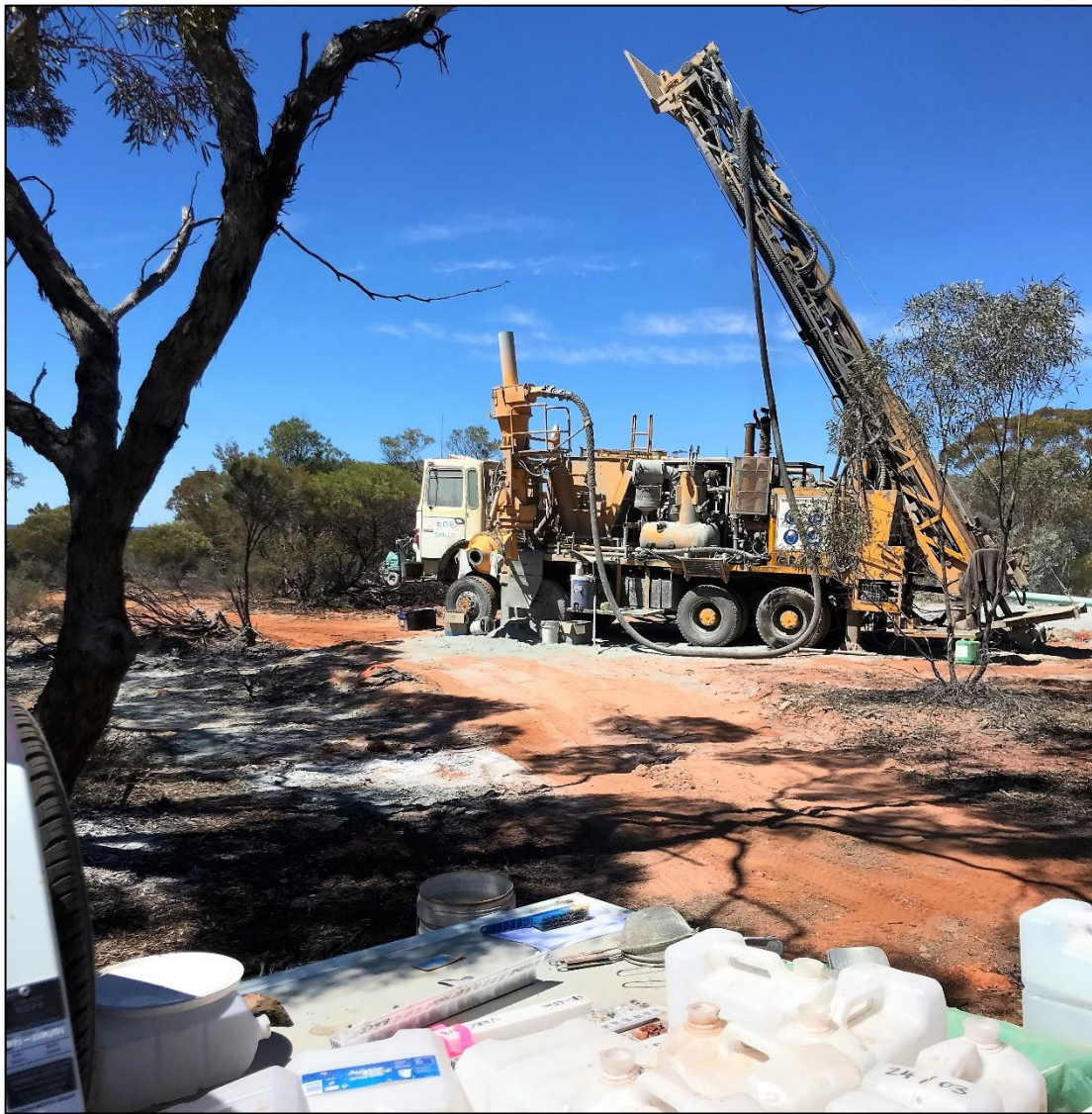
Figure 1; RC drill rig setup on hole VKRC0013 with geologist workstation setup for chip sampling in the back of a ute in the foreground.
