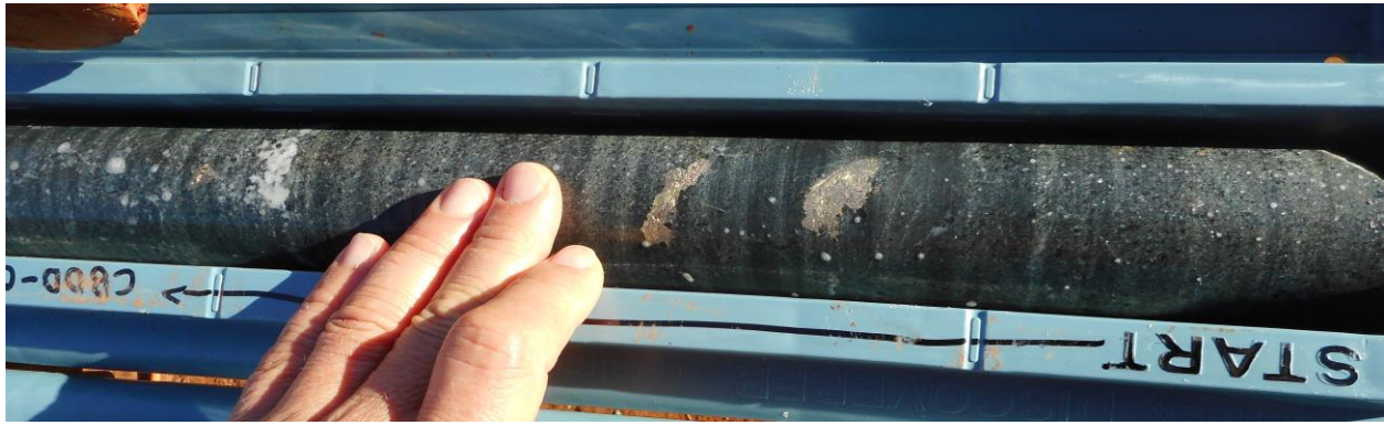
Figure 4: Fragments of nickel-copper sulphides wrapped in clasts of, at the time, semi-solid basal chill zone.
