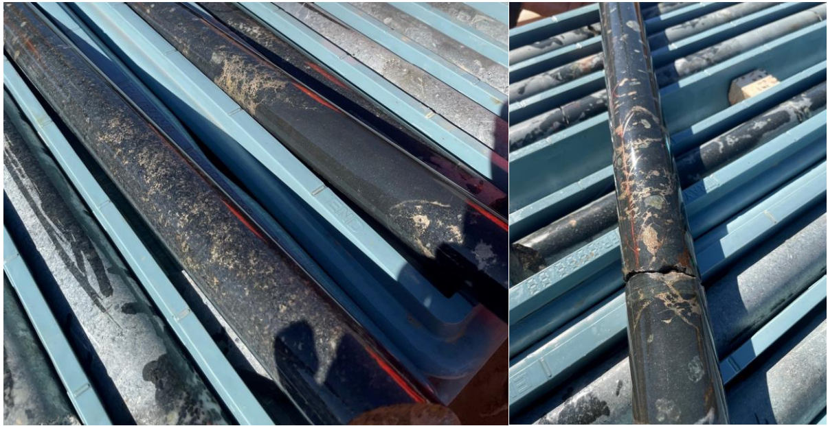
Figure 5: Disseminated and matrix breccia nickel sulphides in CBDD056 at 732m down hole.
