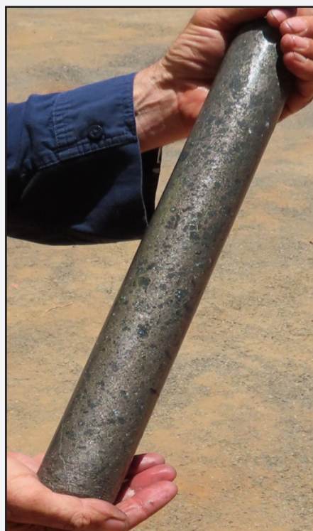
Figure 7: ANDD0006 drill core Massive Ni-Cu sulphides @ 416.9m-417.3m 0.75m @ 3.75% Ni and 0.21% Cu
