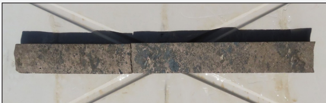
Figure 8: ANDD0011 at VC-23; semi-massive sulphides: 0.67m @ 3.62% Ni & 0.15% Cu
