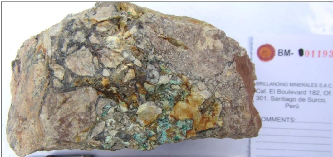
Figure 6: Photo of sample BM-01193 which contains 2,238\text{g/t} Ag (the highest Ag value to date at greater Riqueza). It is a brecciated and highly altered volcanic with visible copper mineralisation. As well as bonanza-grade silver, the sample contains 0.15\% copper and 0.66\% lead.
