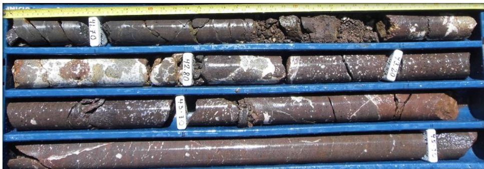
Figure 2: Core photo RDDH025, 41.5m to 45.2m showing highly brecciated iron-oxide altered andesitic sill with visible malachite (copper) mineralisation.
