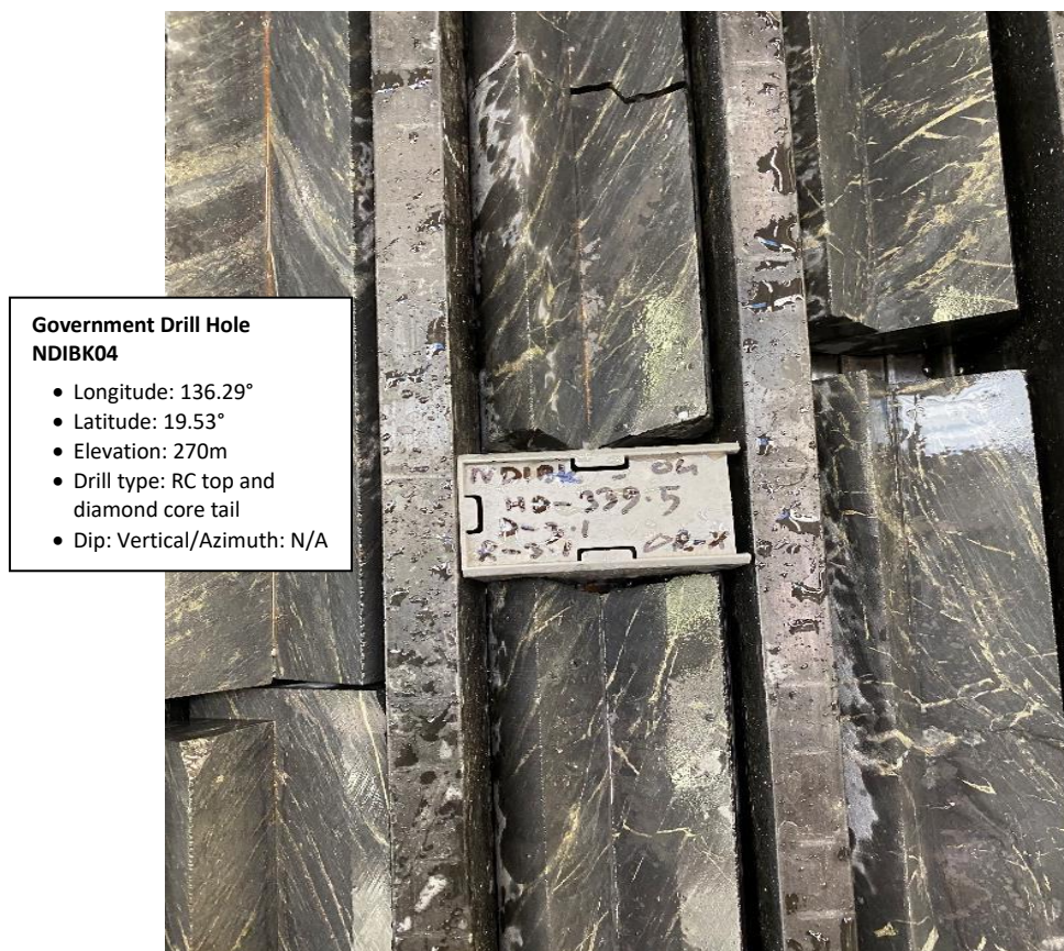
Figure 11: Photo of core from Government drill-hole NDIBK04, core depth is 339.5m. The core has been cut in half and one half has been cut again. A quarter-core sample every metre has been submitted for multi-element analysis. DRILLING WAS NOT CONDUCTED BY INCA.
