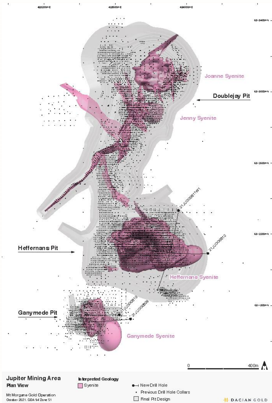
Figure 1: Plan view of the Jupiter syenite complex with the current final pit design
