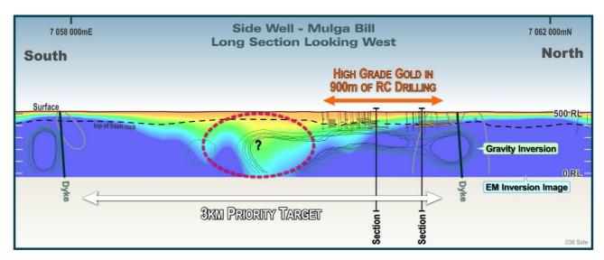
FIGURE 4: LONG SECTION THROUGH MULGA BILL. THE EM HEAT MAP AND GRAVITY CONTOURS HIGHLIGHT THE DEPTH POTENTIAL SOUTH OF CURRENT RC DRILL COVERAGE.
