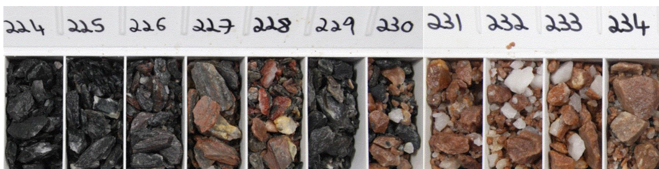
Photo 1: Hole #178 10m @ 5.49g/t Au (from 224m) - Incl. 4m @ 12.49g/t Au (from 228m) RC Hole ended in altered quartz porphyry, diamond drill rig now positioned over this hole to drill ~50m tail
