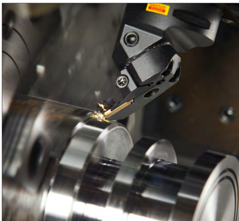
Figure 10 . Tungsten carbide cutting tool.
