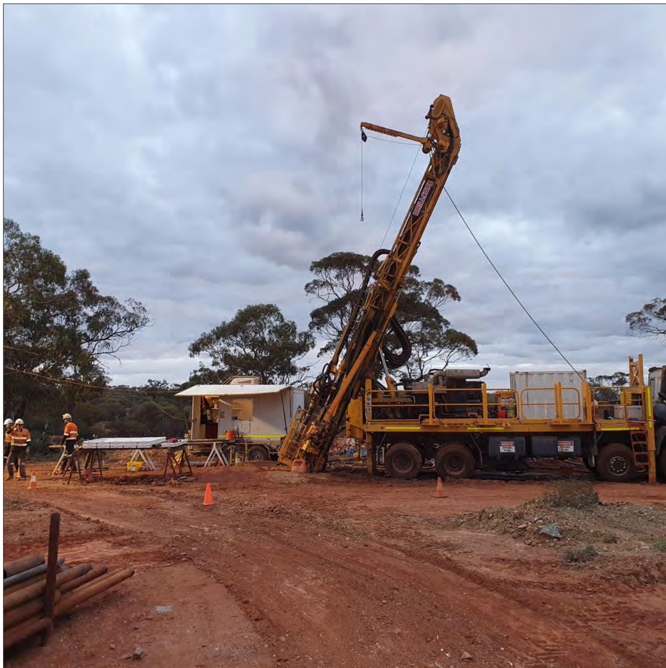
Figure 2. PQ metallurgical drilling underway at Mt Mulgine
