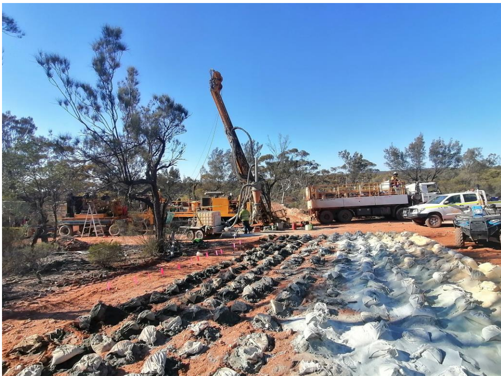
Figure 5: TDA Multipurpose RC Diamond Rig drilling CBP076.
