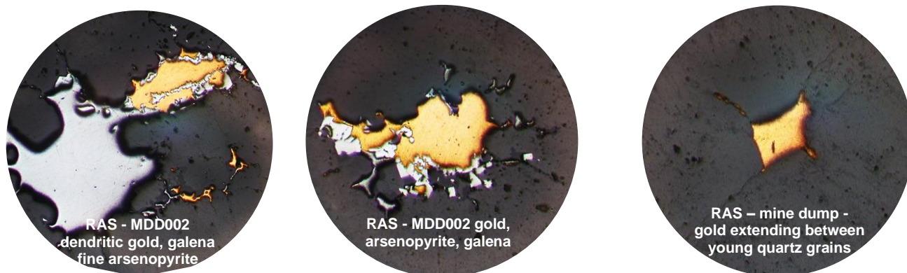
Figure 7 Polished thin section images of gold (field of view ~1mm - PanterA Geoservices)
