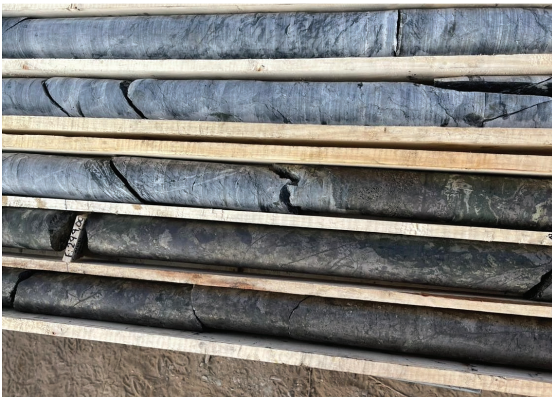
Photo 8 – GNDD-314 Footwall Zone mineralisation from 297-300 metres (2.8m at 62.5 g/t AuEq)
