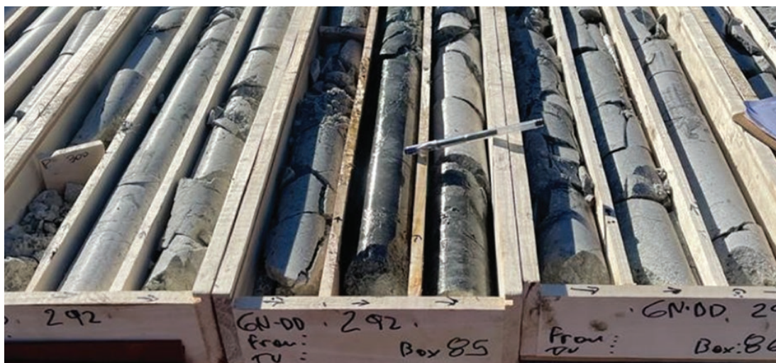
GNDD-292 sulphide interval 233 metres downhole (skarn alteration 15% pyrite 5% sphalerite)
