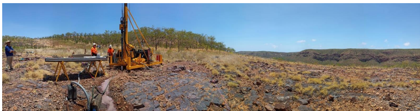
Figure 1. Harmec Drilling heli-portable diamond drill rig set up and drilling at drill hole YMP002D - looking west.
