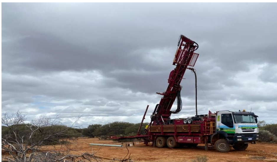
Photo: Reverse Circulation drill rig on site at the Brandy Hill South Project
