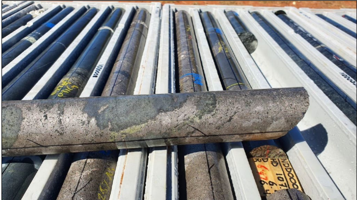
Figure 9. Semi-massive sulphide from approximately 106m downhole in NDD0008, showing the interaction of the sulphides with country rock xenoliths, and clots of remobilised chalcopyrite.
