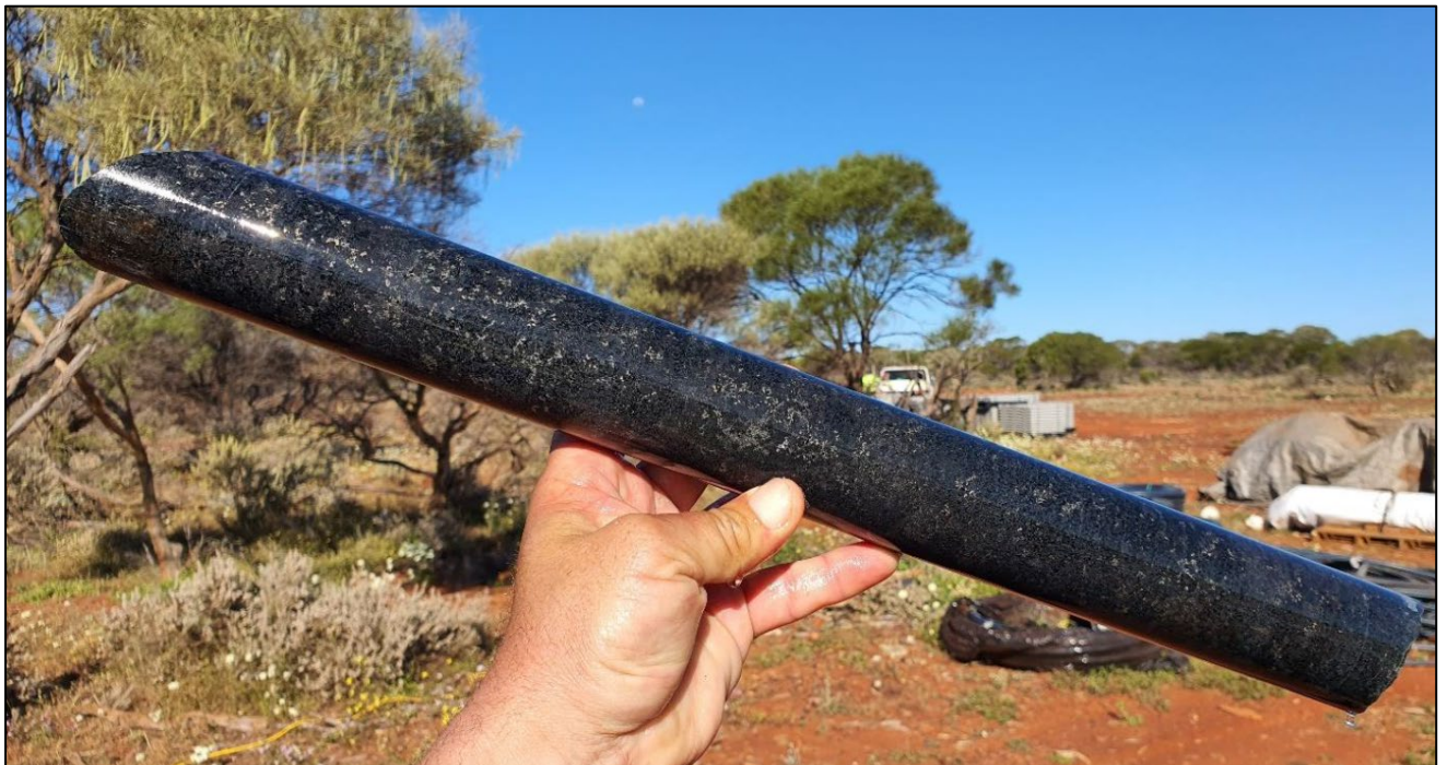
Figure 8. Cumulate-textured high-MgO ultramafic with disseminated and bleby magmatic sulphides from 89m in NDD0008.
