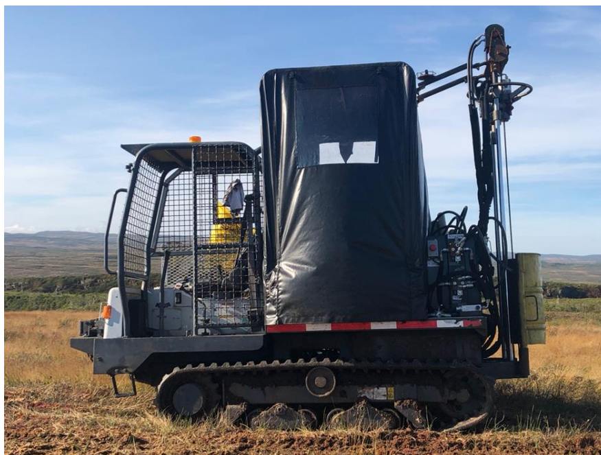
Figure 8: Power auger (rubber track-mounted “Winkie Rig” Mk2)
