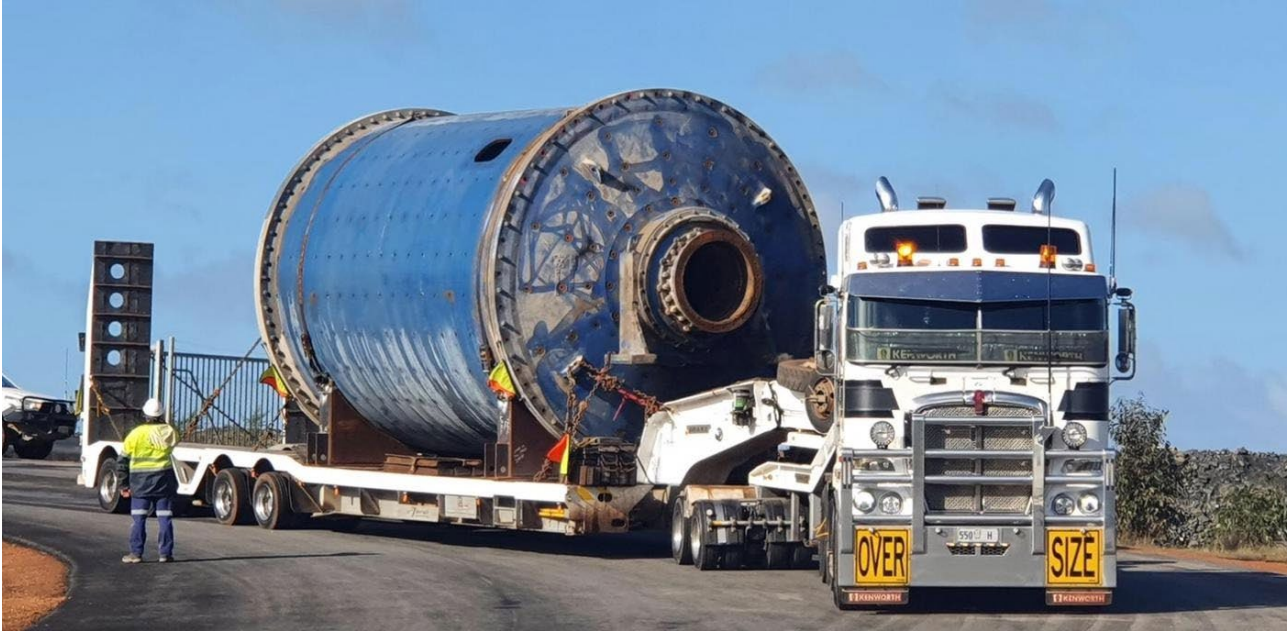
Figure 8: 1.85MW Outokumpu ball mill on the road to Kalgoorlie
